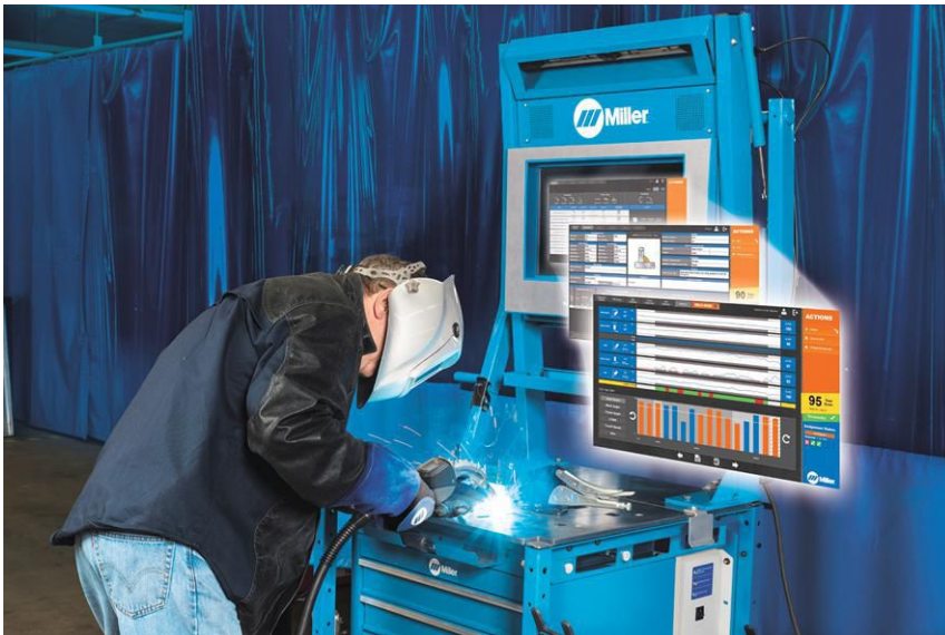
Miller’s LiveArc AR training system gives manual welders accurate, real-time feedback on their work angle, travel angle, contact-tip-to-work distance, travel speed and aim, both during actual welding (as shown here) and in simulation mode. (Provided by Miller Electric Mfg)
