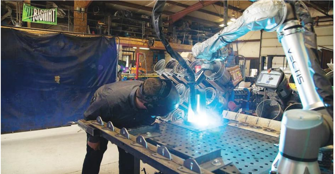
Cobots are a good fit for simpler, repetitive jobs that would bore a human welder, and they can work in close proximity to people. (Provided by Universal Robots)
